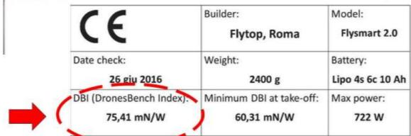
DronesBench Index (DBI) indicates the power efficiency of the drone as a whole.
