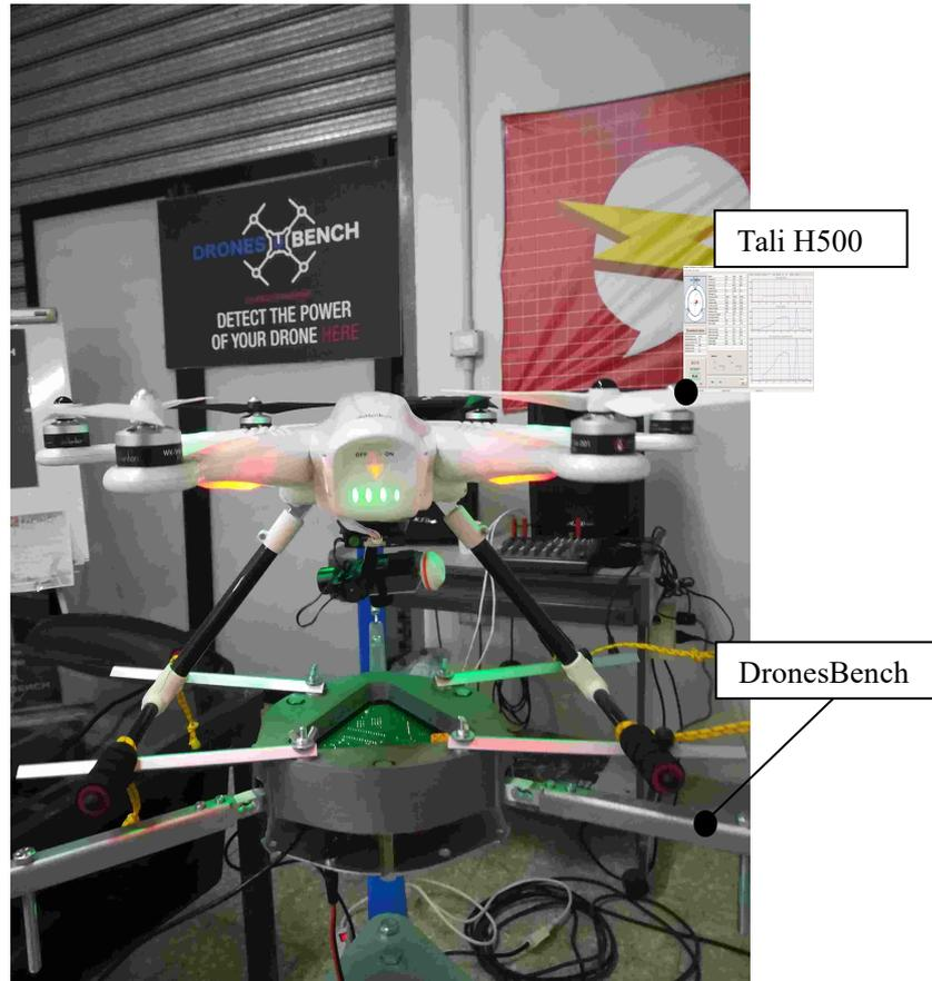
Figure 1: Fixing the drone to the DronesBench before the test
