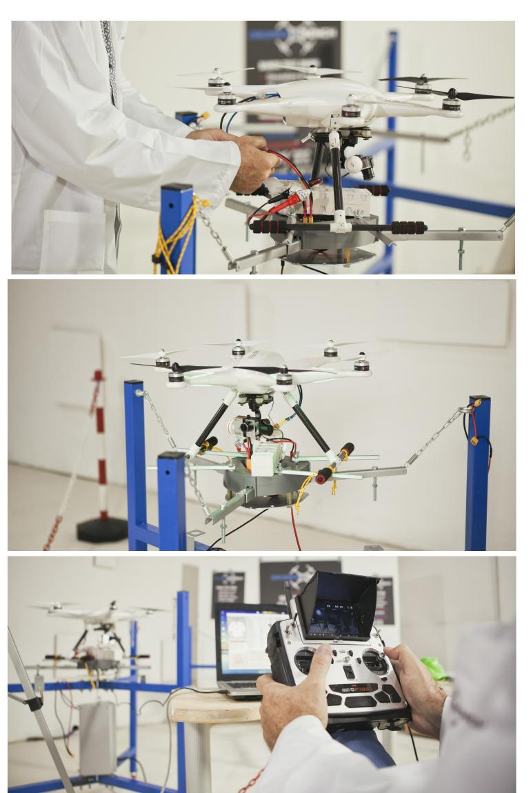
The DronesBench is able to measure contemporarily and without disassembling the drone: (i) the thrust provided by the drone, (ii) the instantaneous power consumption of the drone, and (iii) the pitch, yaw, and roll instantaneous angles during the test.
